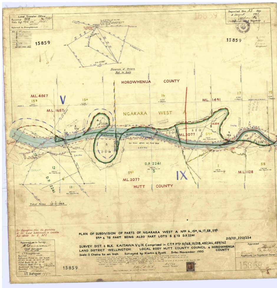
Figure 7 This survey of Parts of Ngarara West A demonstrates why the question of the river boundary was the subject of debate. It demonstrates the centre line of the river by the 1892 survey, compared to its change in 1951. Wellington Plan DP 15859 (Source: Quick maps)
