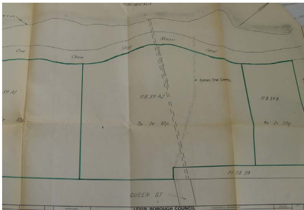
Figure 5.6: Undated borough council plan showing ‘existing open channel’ and ‘proposed open stormwater channel’ (in bolder lines) running through Horowhenua 11B 39 and 11B 39 A2 1162
